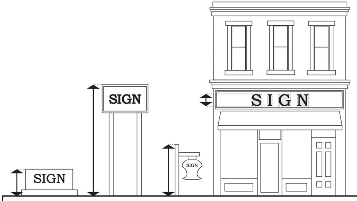
3. Vertical Clearance. For signs attached to a structure, vertical clearance is measured as the vertical distance from the sidewalk or nearest ground level to the lowest point of the sign.
