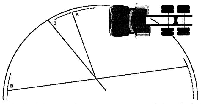
Tests have shown that the true location of the turning center is further to the rear than midway between drive axle sets (where applicable)
