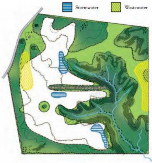
Step 1: Delineate prime soils, natural, historic, and cultural resources, stormwater and wastewater locations and potential development area
